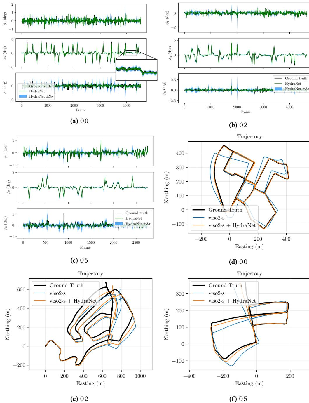
**Figure 7.11:** Results for KITTI sequences 00, 02 and 05. Top-down trajectory plots show localization improvements after fusion with a classical stereo visual odometry pipeline.
