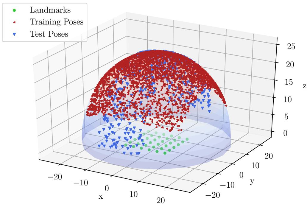
(a) Synthetic world used to illustrate our method. A monocular camera observes a  $6 \times 6$  grid of point landmarks from poses sampled on a semi-sphere. The test set includes poses that are outside the training distribution.
