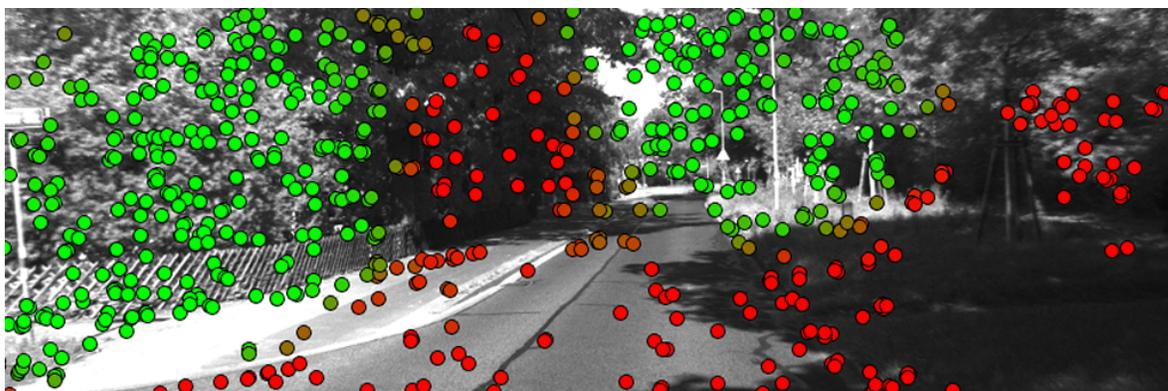
**Figure 4.7:** A high-frequency predictor can distinguish between regions of high and low texture such as foliage and shadows. Green indicates higher values.
