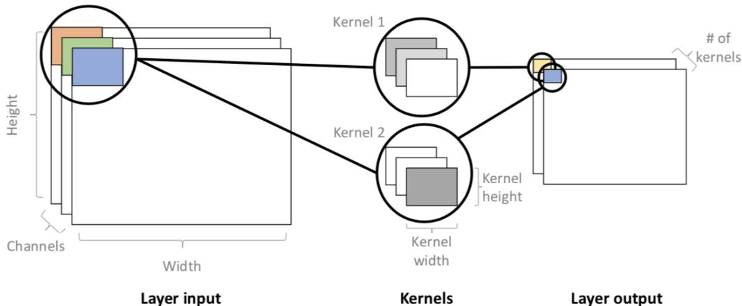
**Figure 2.3:** A convolutional layer with two kernels that operate over different channels of a two-dimensional input. Figure from Gal (2016).
