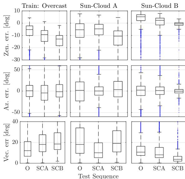
**Figure 5.17:** Box-and-whiskers plot for zenith, azimuth and vector angle errors for nine different combinations of train-test sequences taken from the Oxford Robotcar dataset. Each column corresponds to a different training sequence, and each plot contains three different test sequences. In the bottom legend, we use the labels O: *Overcast*, SCA: *Sun-Cloud A*, SCB: *Sun-Cloud B*.
