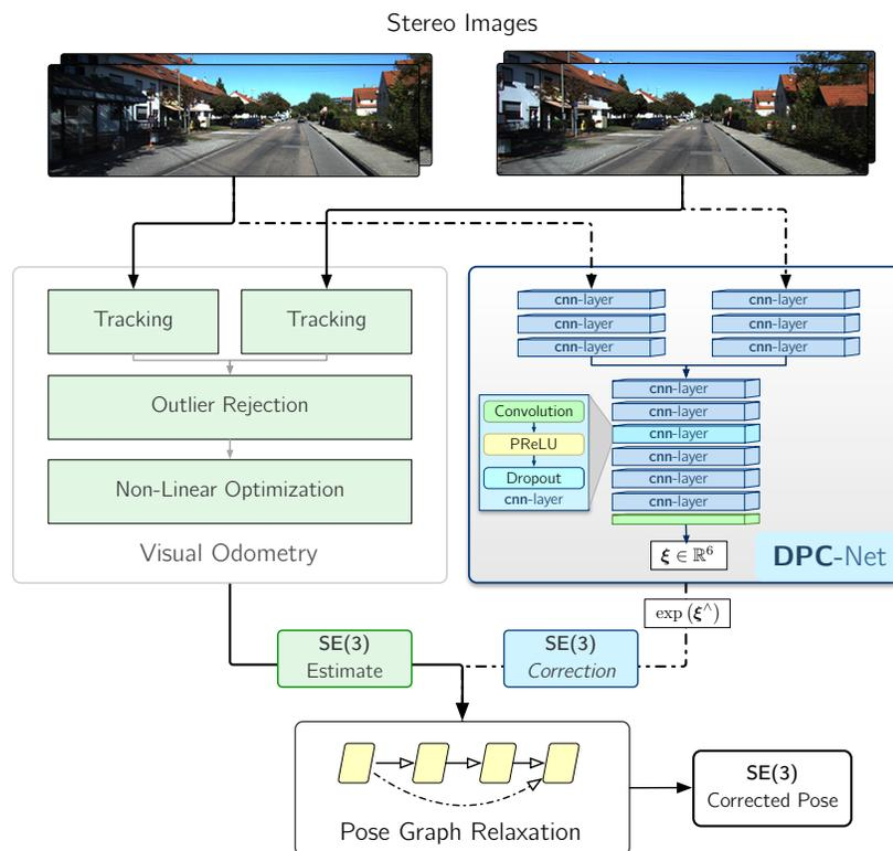
**Figure 6.1:** We propose a Deep Pose Correction network (DPC-Net) that learns  $SE(3)$  corrections to classical visual localizers.
