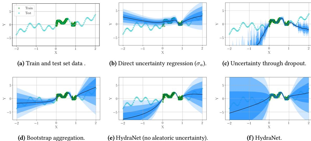
**Figure 7.4:** A comparison of different ways to extract uncertainty from deep networks. Each shade of blue represents one standard deviation  $\sigma$  produced by the model.
