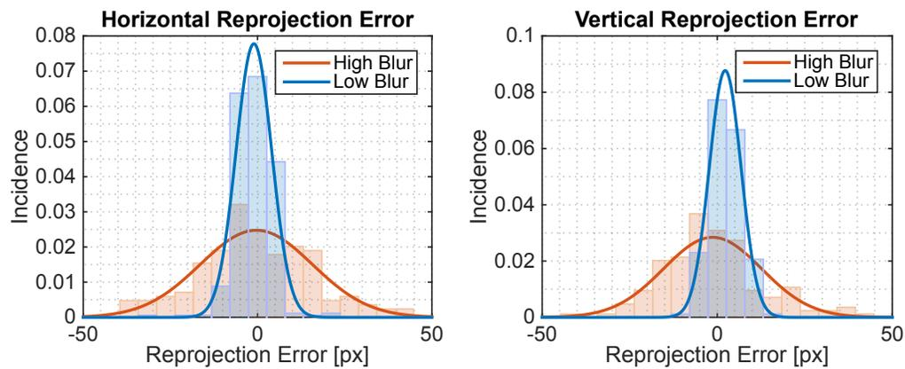
**Figure 4.4:** Reprojection error of checkerboard corners triangulated from the VI-Sensor and reprojected into the Flea3. We distinguish between high and low blur by thresholding the blur metric [Crete et al. \(2007\)](#).
