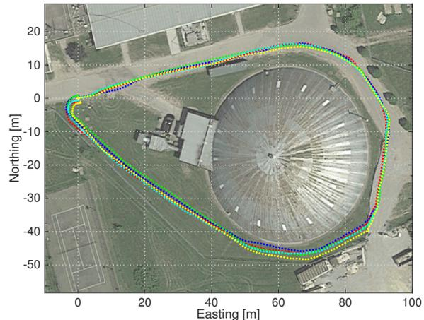
(b) GPS ground truth for 5 experimental trials collected near the UTIAS Mars Dome. Each trial is approximately 250 m long.
