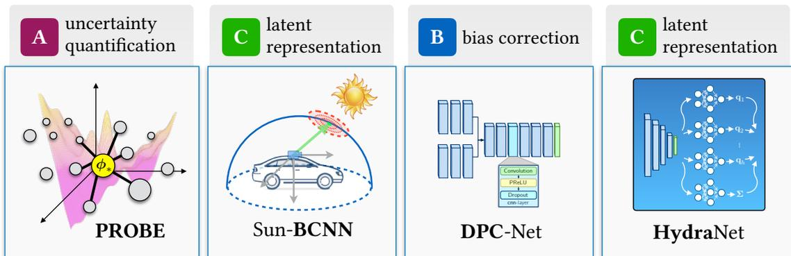
**Figure 1.6:** We present four data-driven models that quantify uncertainty (PROBE), correct bias (DPC) and independently extract latent quantities such as sun direction (Sun-BCNN) and relative rotation (HydraNet).
