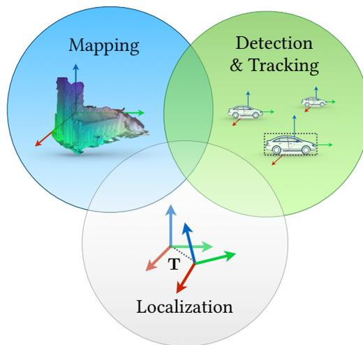
**Figure 1.2:** A Venn diagram depicting three major components of visual perception in the context of mobile autonomy. Egomotion estimation is a form of self-localization that can aid both mapping and detection.
