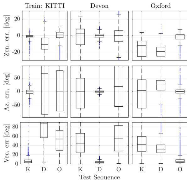
**Figure 5.18:** Box-and-whiskers plot for zenith, azimuth and vector angle errors for nine different combinations of train-test datasets. Each column corresponds to a different training sequence, and each plot contains three different test sequences. In the bottom legend, we use the labels K: KITTI, D: Devon Island, O: Oxford. All three models produce large biased errors when applied to other datasets, likely due to variations in optical properties and parameter settings across cameras.
