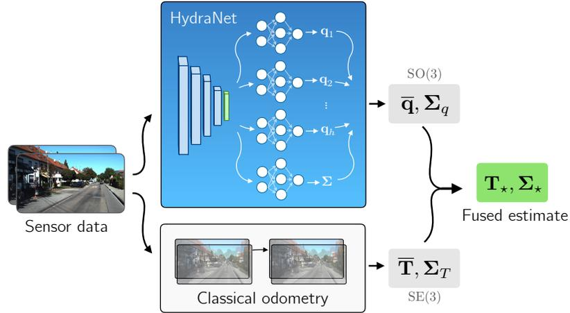
**Figure 7.1:** HydraNet produces an estimate of relative rotation (with a principled covariance matrix) that can be fused with existing egomotion pipelines through pose graph optimization.
