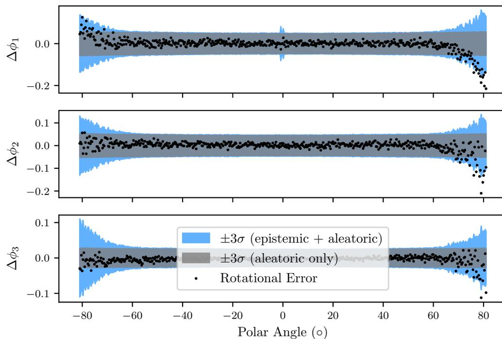
(b) Rotation estimation errors for a deep network trained using our HydraNet approach on synthetic data (noisy pixel locations of 36 landmarks). We note that outside of the training distribution, our epistemic uncertainty ( $\Sigma_e$ ) grows, as expected.
