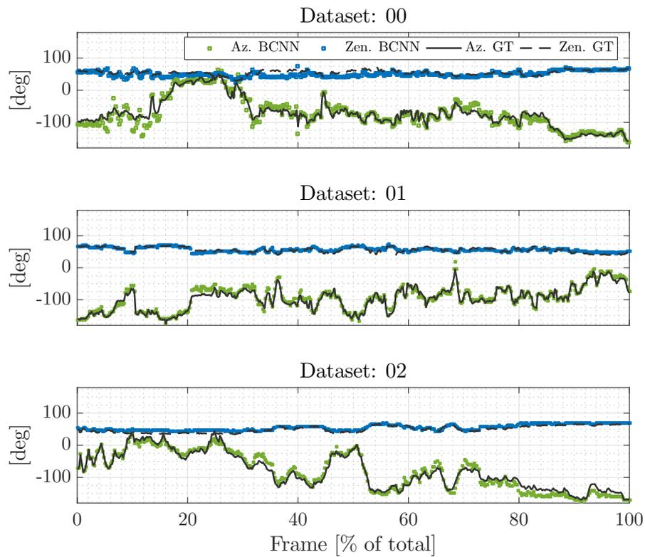
**Figure 5.12:** Azimuth (Sun-BCNN azimuth and zenith predictions over time for Devon Island test sequences 00, 01 and 12. Sun-BCNN is trained and tested on all frames (in our VO experiments, we use the Sun-BCNN predictions of every tenth image to make a fair comparison).
