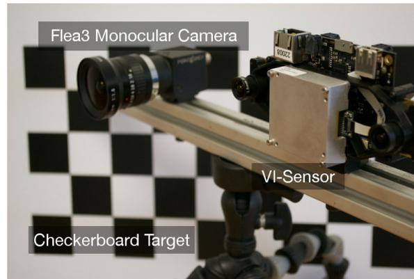
**Figure 4.3:** The Skybotix VI-Sensor, Point Grey Flea3, and checkerboard target used in our motion blur experiments.
