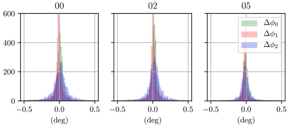
**Figure 7.12:** Error histograms for test KITTI sequences 00, 02, and 05 on three rotational axes.
