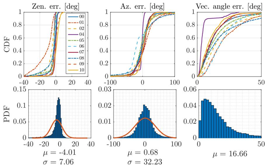
**Figure 5.5:** Distributions of azimuth error, zenith error, and angular distance for Sun-BCNN compared to ground truth over each test sequence in the KITTI dataset. *Top row:* Cumulative distributions of errors for each test sequence individually. *Bottom row:* Histograms and Gaussian fits of aggregated errors.
