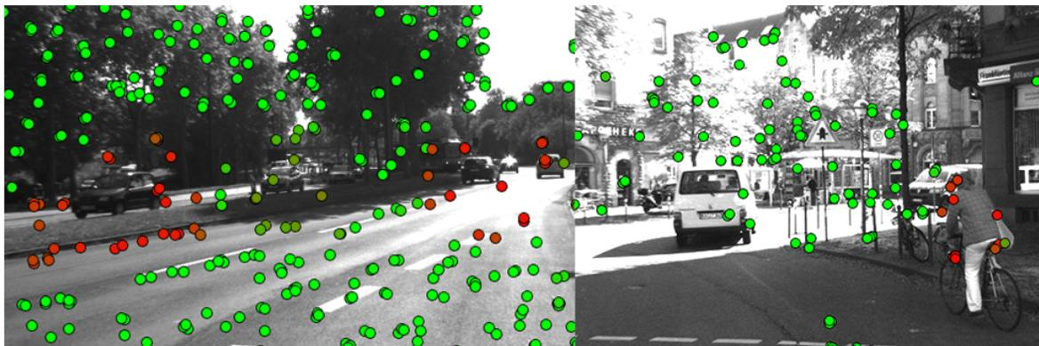
**Figure 4.6:** The optical flow variance predictor can help in detecting moving objects. Red circles correspond to higher values of the optical flow variance score (i.e., features more likely to belong to a moving object).
