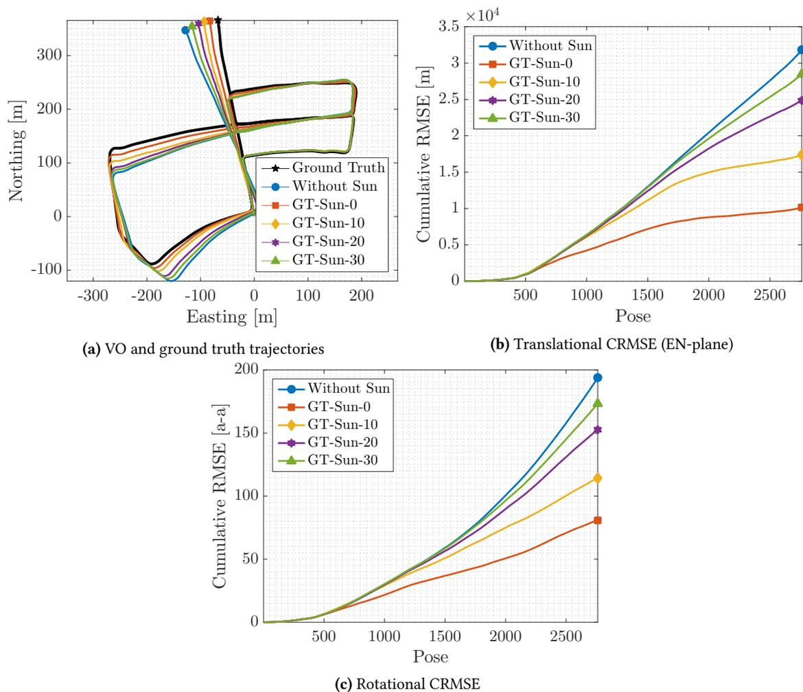
**Figure 5.8:** VO results for KITTI odometry sequence 05 using simulated sun measurements at every tenth pose. We observe a clear progression in cumulative root mean squared error (CRMSE) in translation and rotation as noise in the simulated sun measurements increases.
