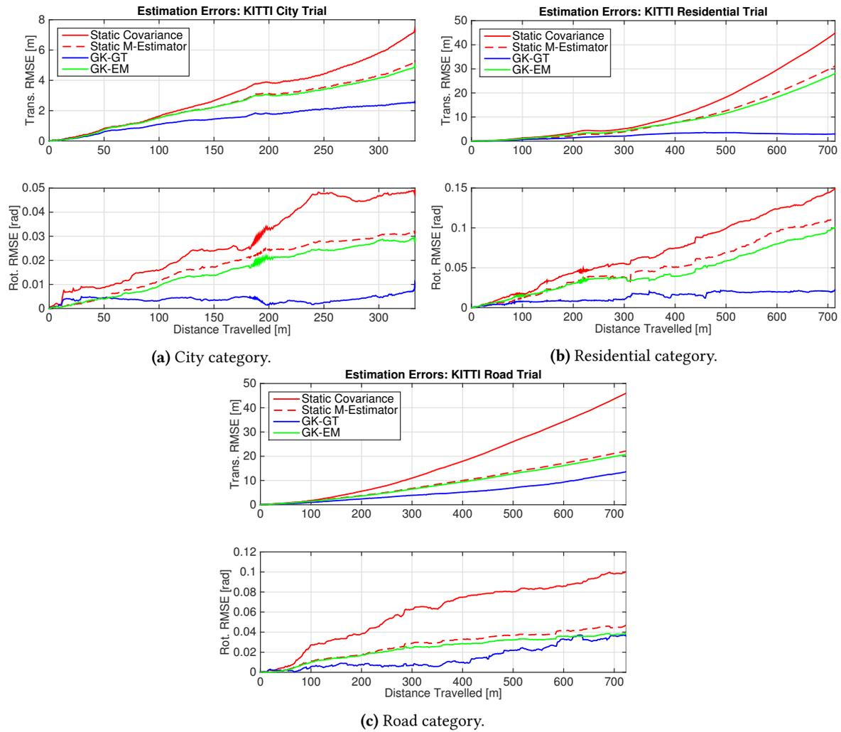
**Figure 4.11:** RMSE comparison of stereo VO estimators evaluated on data in the KITTI odometry benchmark. See Table 4.1 for a quantitative summary.
