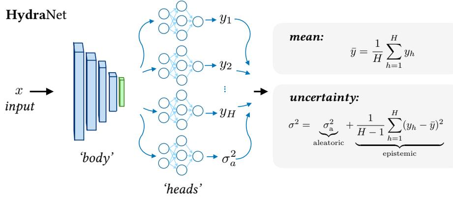
**Figure 7.2:** The HydraNet structure. Input data is passed through a main body and then through a number of heads. Outputs are combined to produce an average and an uncertainty.
