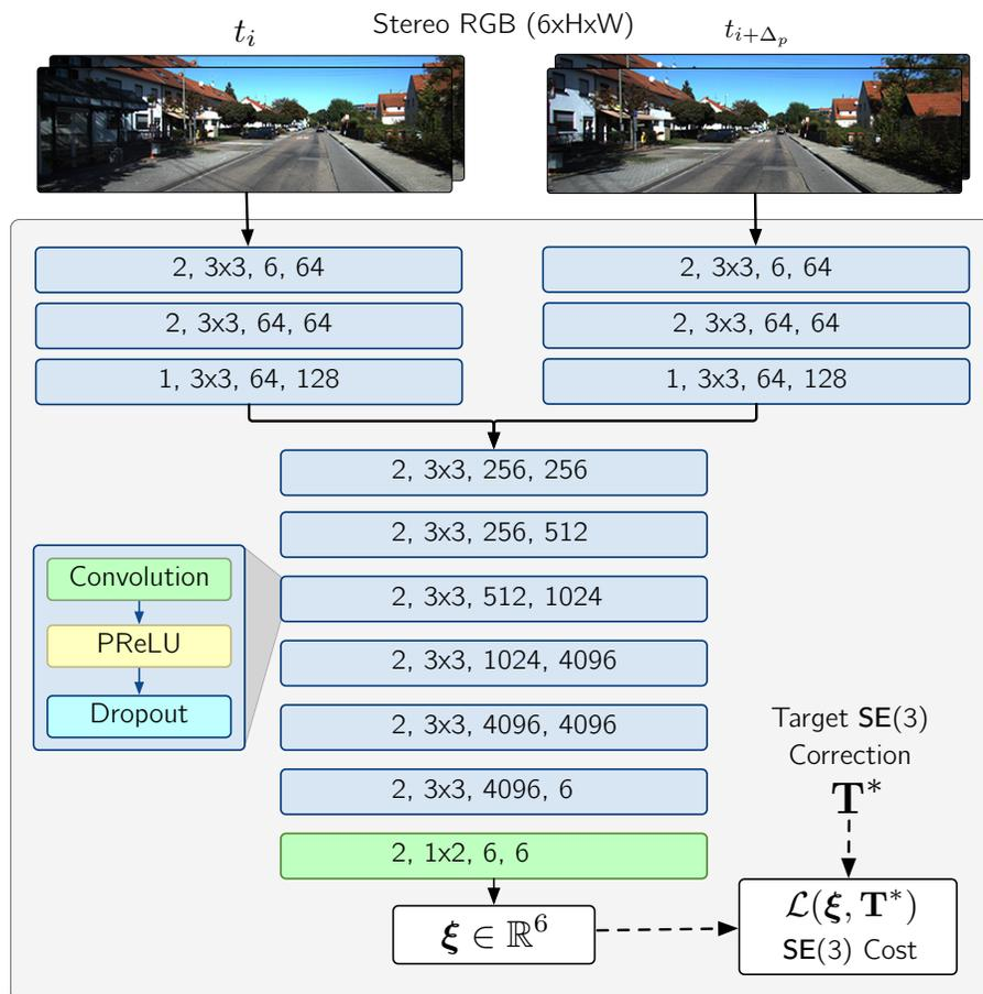
**Figure 6.2:** The Deep Pose Correction network with stereo RGB image data. The network learns a map from two stereo pairs to a vector of Lie algebra coordinates. Each darker blue block consists of a convolution, a PReLU non-linearity, and a dropout layer. We opt to not use MaxPooling in the network, following [Handa et al. \(2016\)](#). The labels correspond to the stride, kernel size, and number of input and output channels of for each convolution.
