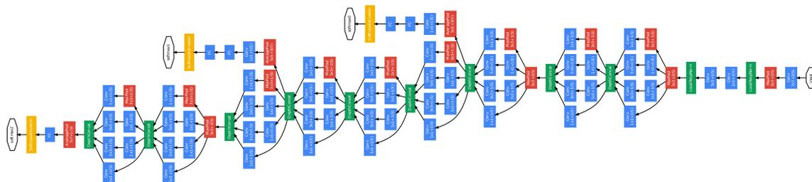
**Figure 5.4:** The GoogLeNet architecture used in this work. This deep convolutional network relies on *inception* modules that concatenate the output of several convolutions with a max-pooling operation. Figure from Szegedy et al. (2015).
