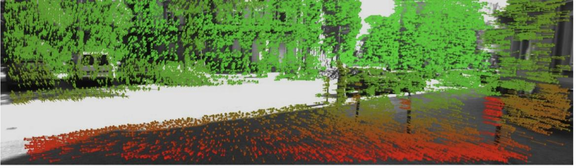
**Figure 3.4:** Feature tracking using viso2, taken from [Geiger et al. \(2011\)](#). Colours correspond to depth.
