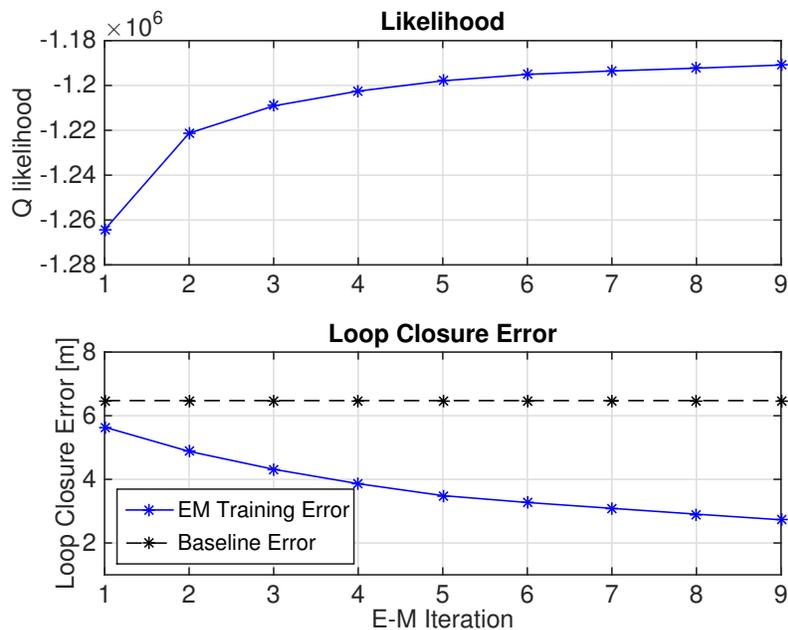
**Figure 4.13:** Training without ground truth using PROBE-GK-EM on a 250.2m path around the Mars Dome at UTIAS. The likelihood of the data increases with each iteration, and the loop closure error decreases, improving significantly from a baseline static M-estimator.
