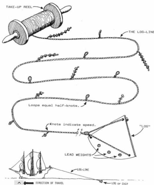
**Figure 1.1:** A *chip log* is a historical tool used to measure ship speed. The *log* or *chip* was tossed into the water, and speed was measured by the amount of *knots* that unravelled in a set time interval (credit: [oceanmotion.org](http://oceanmotion.org)).
