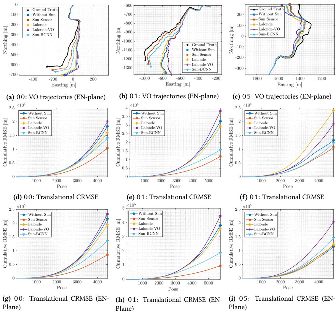
**Figure 5.15:** VO results for Devon Island sequences 00, 01, and 05 using estimated sun directions. *Top row:* Estimated and ground truth trajectories in the EN-plane. *Bottom rows:* Translational cumulative root mean squared error (CRMSE). Sun-BCNN significantly reduces the estimation error on sequences where the sun sensing has an impact (c.f. ??).
