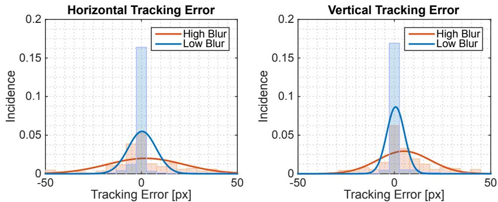
**Figure 4.5:** Effect of blur on reprojection and tracking error for the slow-then-fast checkerboard dataset. We distinguish between high and low blur by thresholding the blur metric [Crete et al. \(2007\)](#). The variance in both errors increases with blur.
