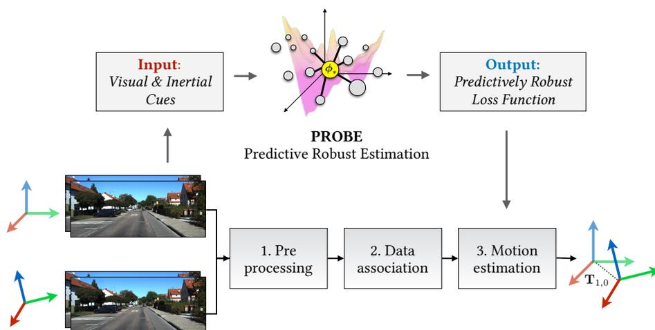
**Figure 4.1:** PROBE builds a predictive noise model for stereo visual odometry.
