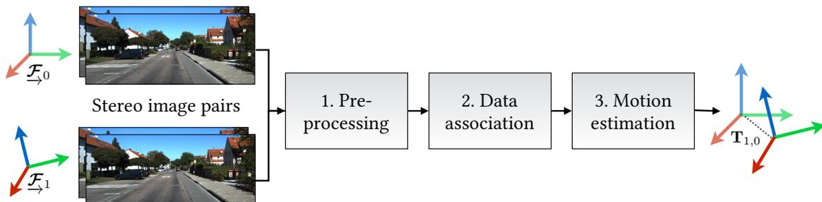
**Figure 3.2:** A ‘classical’ stereo visual odometry pipeline consists of several distinct components that have interpretable inputs and outputs.
