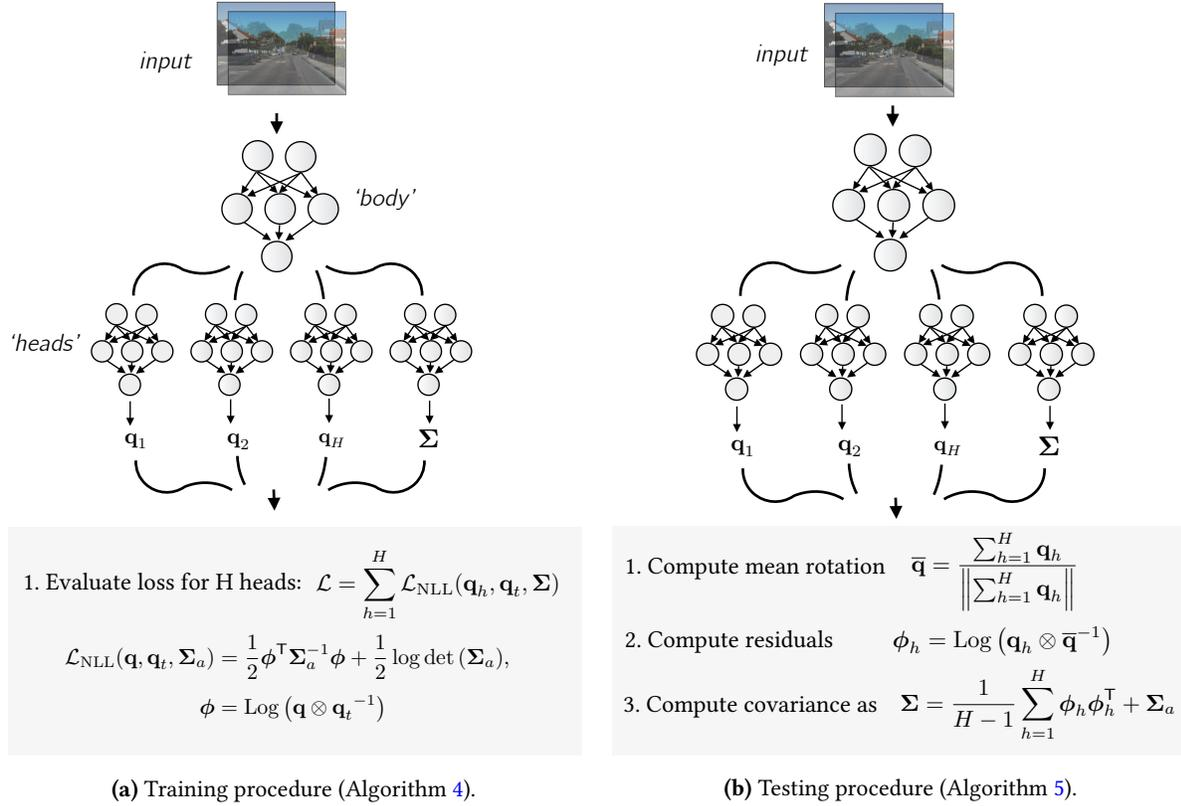
**Figure 7.8:** The training and testing procedures for HydraNet for unit quaternion targets.
