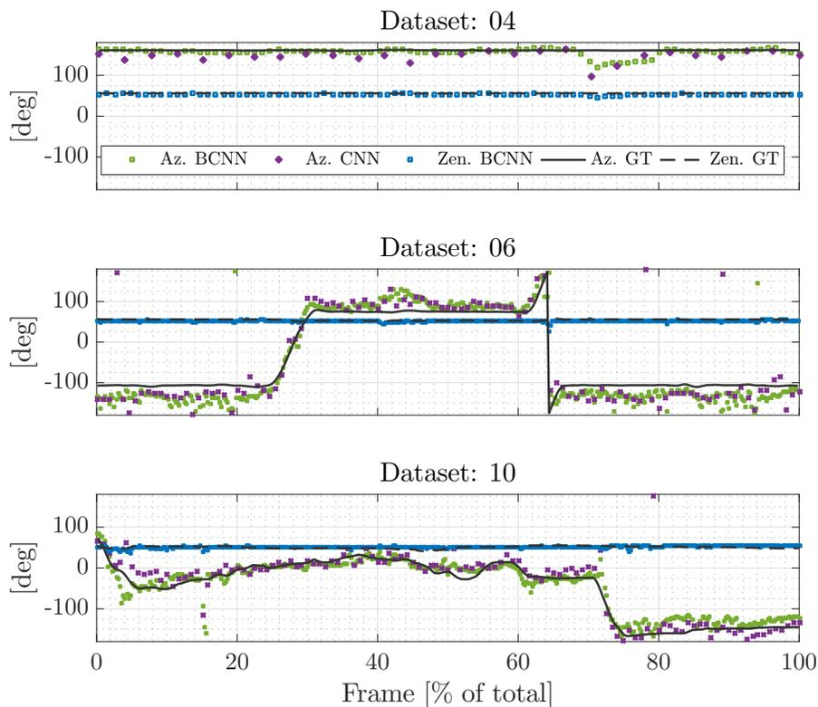
**Figure 5.6:** Azimuth (Sun-CNN and Sun-BCNN) and zenith (Sun-BCNN only) predictions over time for KITTI test sequences 04, 06 and 10. Sun-CNN is trained and tested on every tenth image, whereas Sun-BCNN is trained and tested on every image. In our VO experiments, we use the Sun-BCNN predictions of every tenth image to make a fair comparison.
