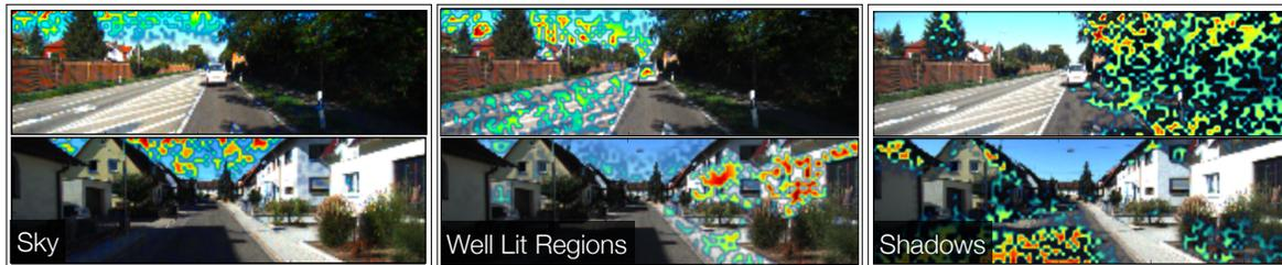
**Figure 5.3:** Three conv1 layer activation maps superimposed on two images from the KITTI odometry benchmark (Geiger et al., 2013) 00 and 04 for three selected filters. Each filter picks out salient parts of the image that aid in sun direction inference.
