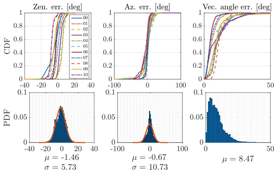
**Figure 5.11:** (Devon Island) Distributions of azimuth error, zenith error, and angular distance for Sun-BCNN compared to ground truth over each test sequence. *Top row:* Cumulative distributions of errors for each test sequence individually. *Bottom row:* Histograms and Gaussian fits of aggregated errors.
