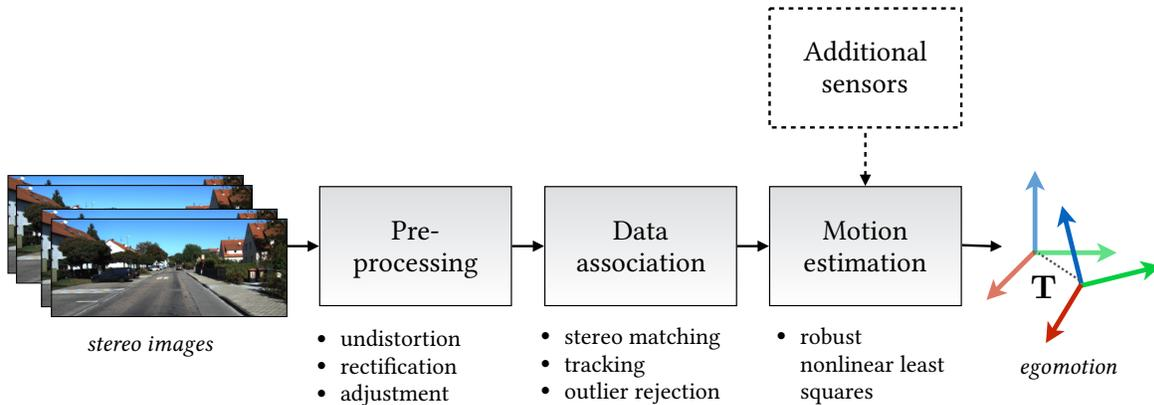
**Figure 1.4:** A ‘classical’ visual odometry pipeline consists of several distinct components with interpretable inputs and outputs. We list common examples of each component.
