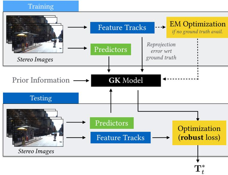
**Figure 4.2:** PROBE builds a predictive noise model using Generalized Kernels (GK) for stereo visual odometry. The model can be trained with and without groundtruth egomotion.
