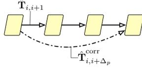
**Figure 6.3:** We apply pose graph relaxation to fuse high-rate visual localization estimates ( $\hat{\mathbf{T}}_{i,i+1}$ ) with low-rate deep pose corrections ( $\hat{\mathbf{T}}_{i,i+\Delta_p}^{\text{corr}}$ ).
