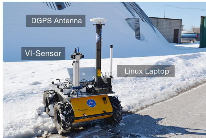
**Figure A.2:** Our four-wheeled skid-steered Clearpath Husky rover equipped with Skybotix VI-Sensor and Ashtech DGPS antenna used to collect the outdoor UTIAS dataset.
