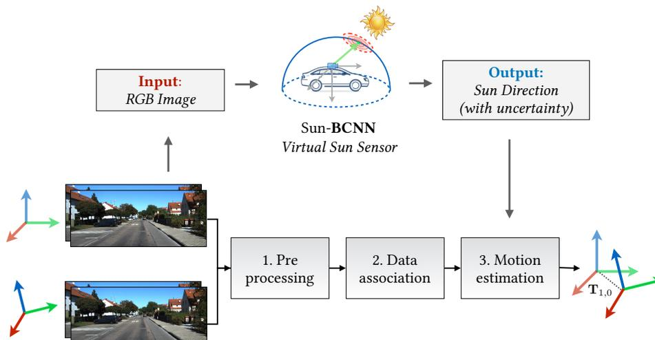
**Figure 5.1:** Sun-BCNN is a learned virtual sun sensor that outputs sun direction with an associated uncertainty based on a single RGB image. We use this as a source of orientation information within a privileged reference frame.
