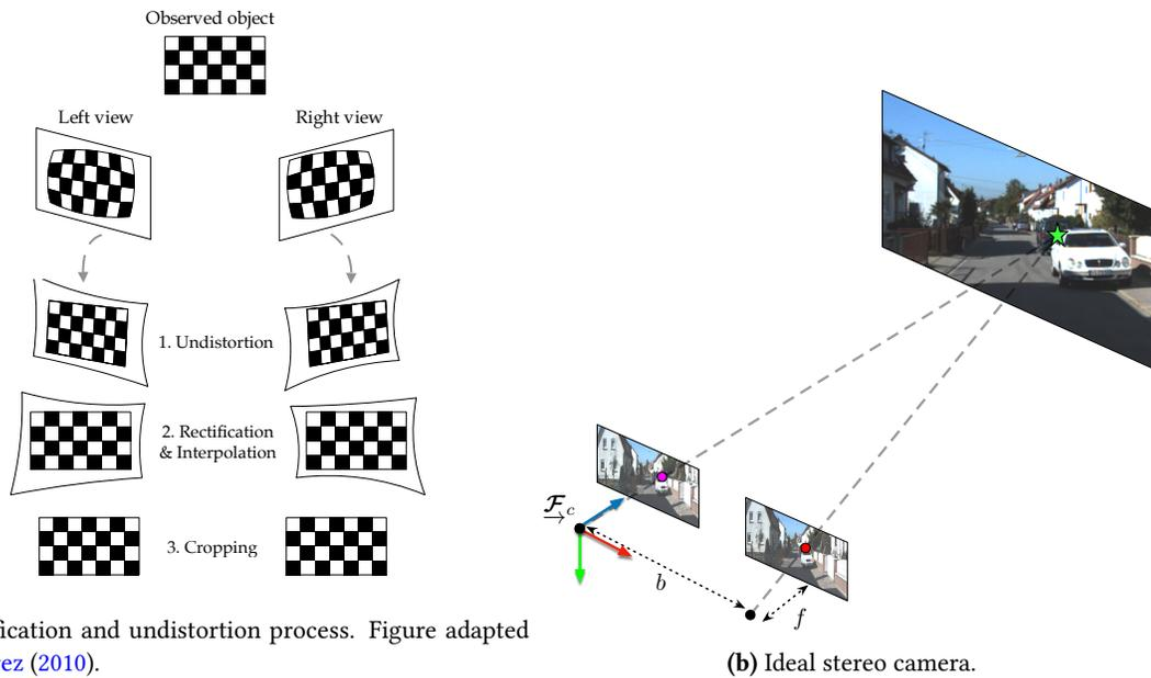
(a) Rectification and undistortion process. Figure adapted from Florez (2010).
