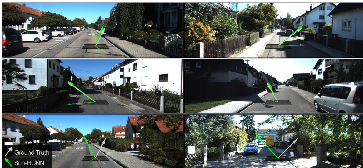
**Figure 5.9:** Sun BCNN predictions and associated ground truth sun directions on the KITTI sequence 05. *Top two rows:* Sun BCNN produces accurate predictions in a variety of azimuth values. *Bottom row:* Poor results occur rarely due to shadow ambiguities.
