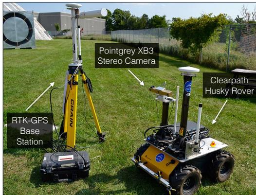
(a) Our experimental apparatus: a Clearpath Husky rover outfitted with a PointGrey XB3 stereo camera and a differential GPS receiver and base station.
