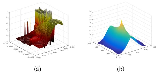
Fig. 2. Example of an augmented *terrain* map using a combination of science parameters along with bathymetry information. Fig. (a) is the resulting terrain map, and Fig. (b) is the auto-correlogram. The data for the figures was collected off Santa Catalina Island, CA.
