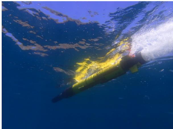
Fig. 1. YSI EcoMapper Autonomous Underwater Vehicle executing a mission off the coast of Santa Catalina Island.
