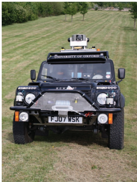
Bowler WildCat autonomous vehicle platform. (Photo courtesy of the University of Oxford Mobile Robotics Group.)
