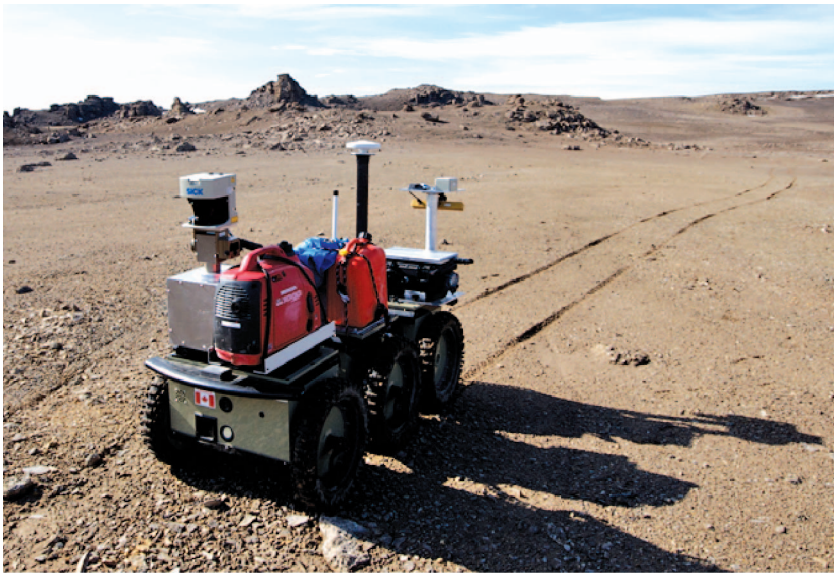
Field robot on Devon Island in 2009 testing long-range autonomous driving in planetary analog domain. (Photo courtesy of Tim Barfoot.)
